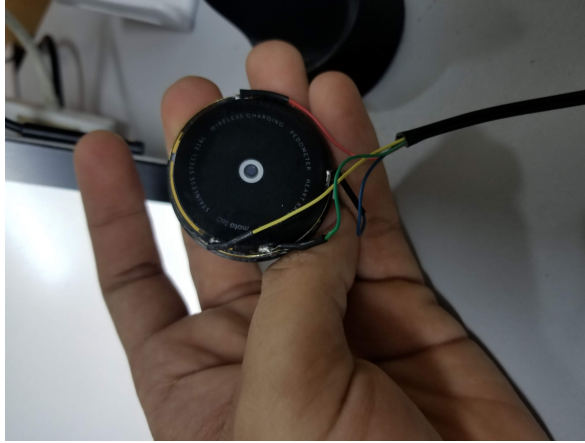
Figure 2.2: The first attempt at soldering on the USB connector, without opening the back.
